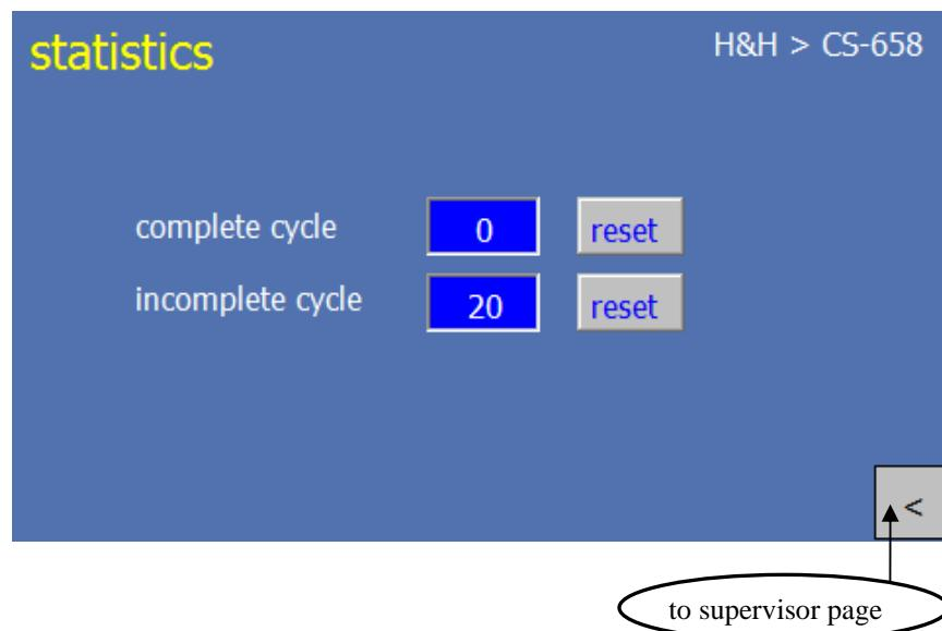
It will show the information of the complete press cycle and incomplete cycle times (triggered by cancel button or safety bar). You can reset both the cycle with the respective reset button. It can prevent the operator from illegally to break the immature cycle for increase the production rate.
