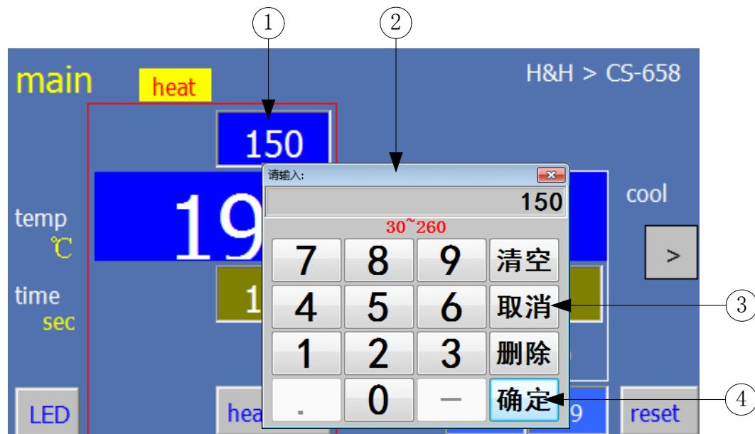
1. heating temperature preset button & display
