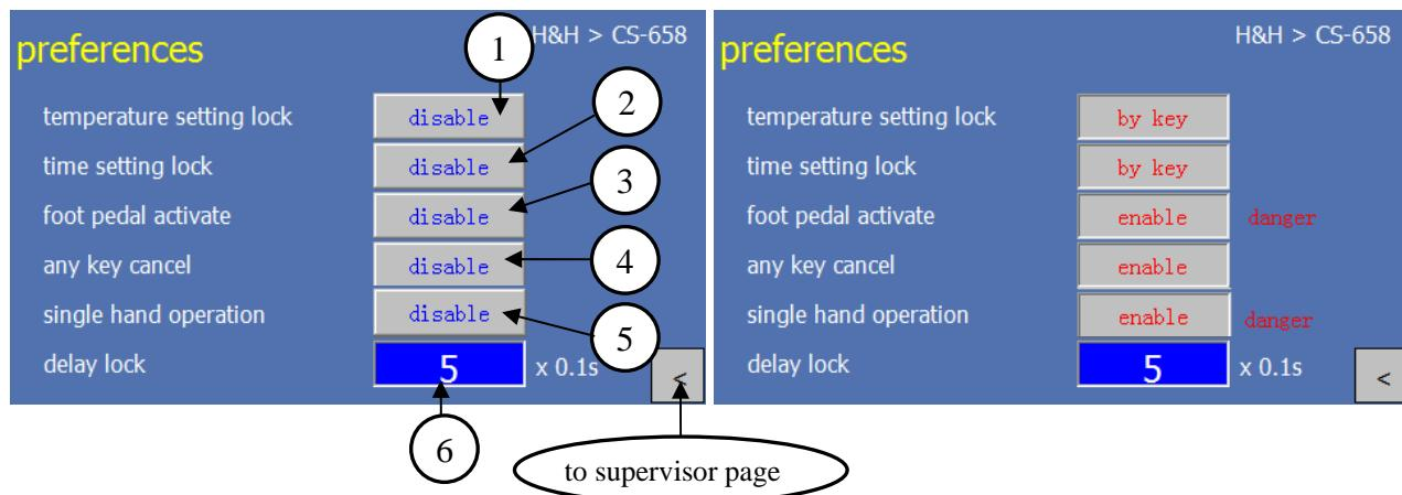
1. press to select the temperature setting lock “off” or “by key”
