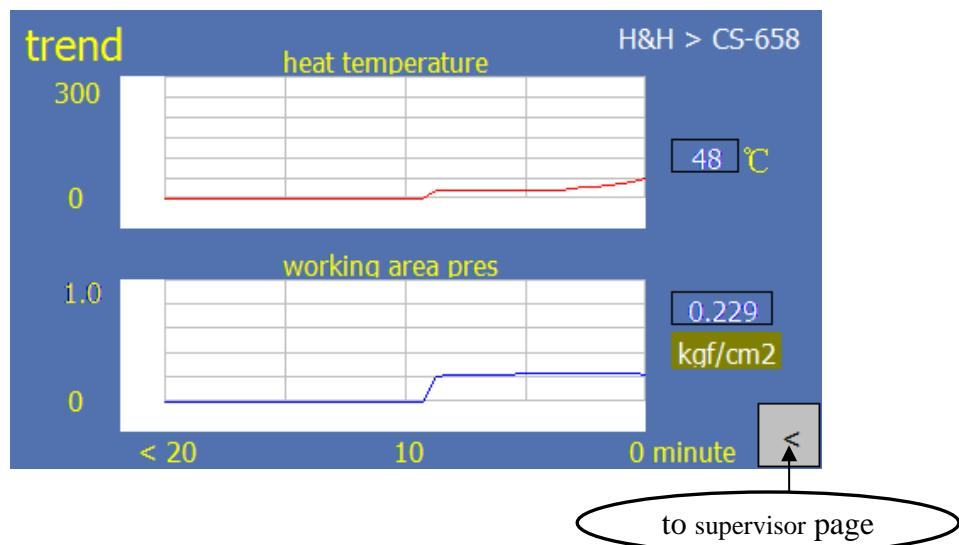
You can check the trend of the working area pressure and temperature in the recent 20 minutes
