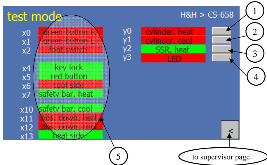
1. press to activate the heat side cylinder
