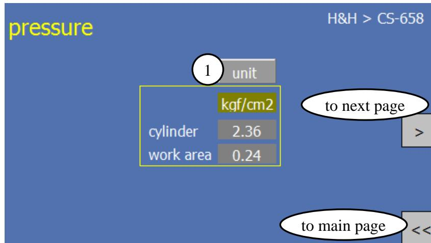
press 1# button you can change the pressure unit (kgf/cm2, MPa, Bar, Psi).
